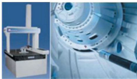
Figure 3: CMM scanner and contact pipalo
