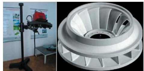
Figure 8: ATOM GOM scanner and scanned Francis turbine rotor
